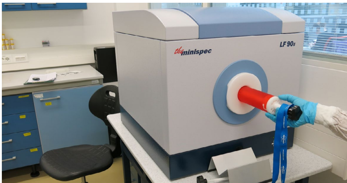
Fig. 1: Body composition analyzer, using the technology quantitative magnetic resonance (TD-NMR), Minispec LF90II, Bruker
