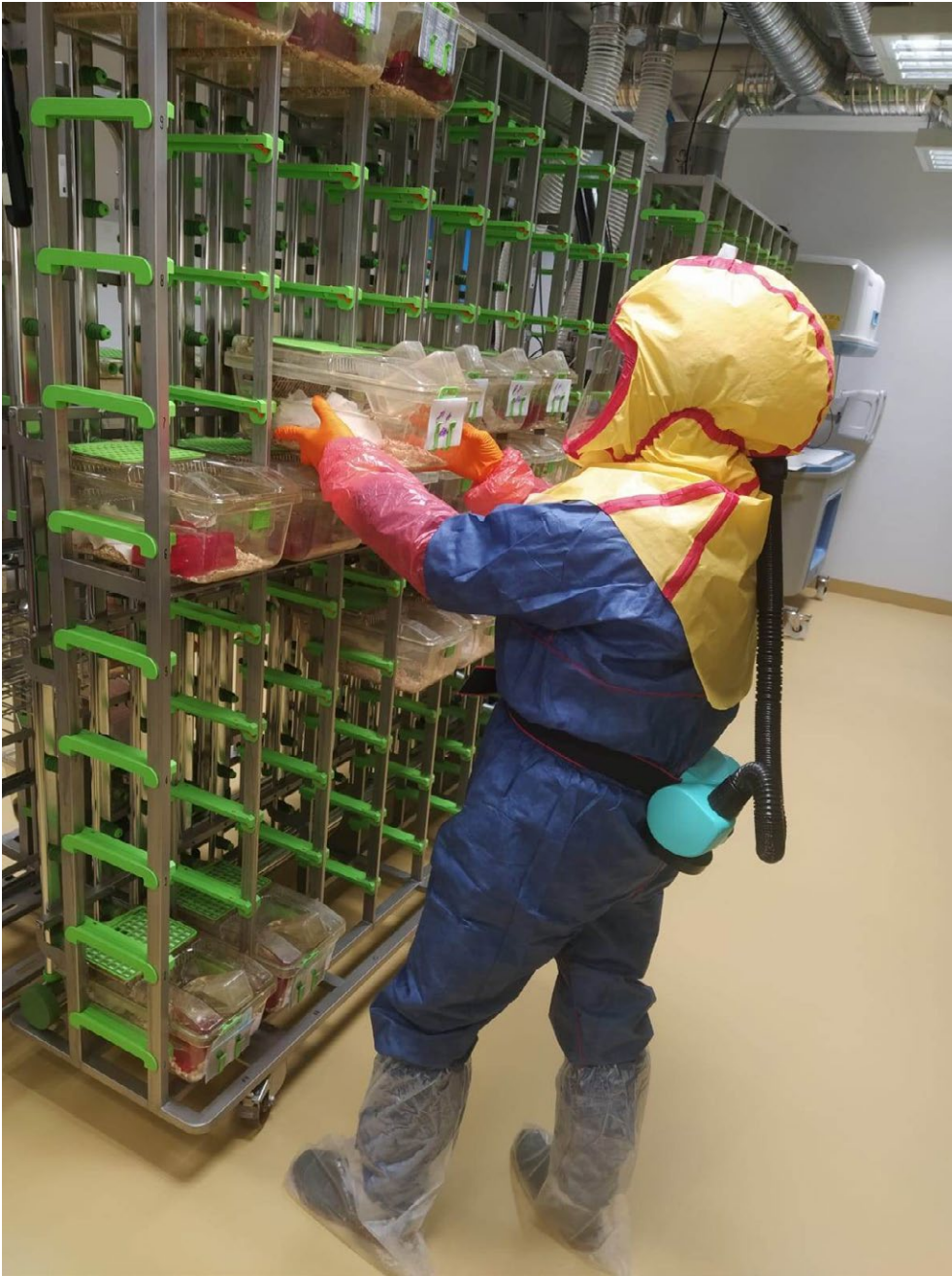
Fig. 1: BSL-3 facility: All animals are housed in IVCs which are connected with Biosafety level 3 ventilation system
